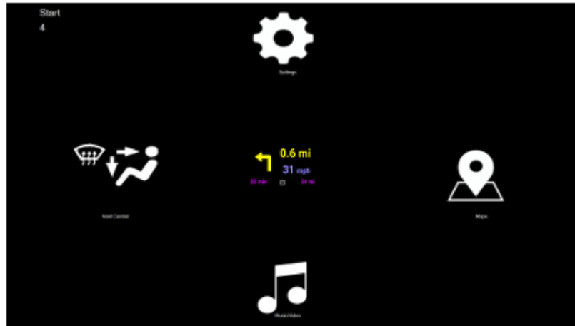
Fig. 3. User Interface Design on Head Up Display
